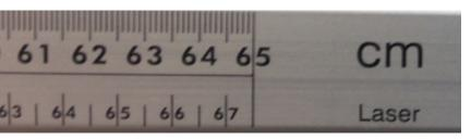
Aim the two perfectly aligned laser pointers as if you were actually at the stem – just pull the caliper jaws apart until the laser points are positioned where you need them to be. Read the diameter results on laser scale if available on your caliper. One inch or 2.54 cm must be added to the regular diameter scale result. If you are using Gator Eyes on a computer caliper from Haglöf (DP II, Digitech® Professional), results can be registered with the press of a button.
